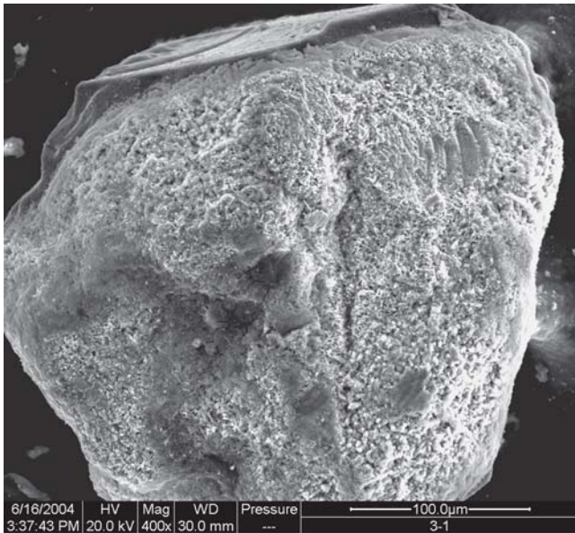
Fig. 4 General micrograph showing the brazed CBN crystal
